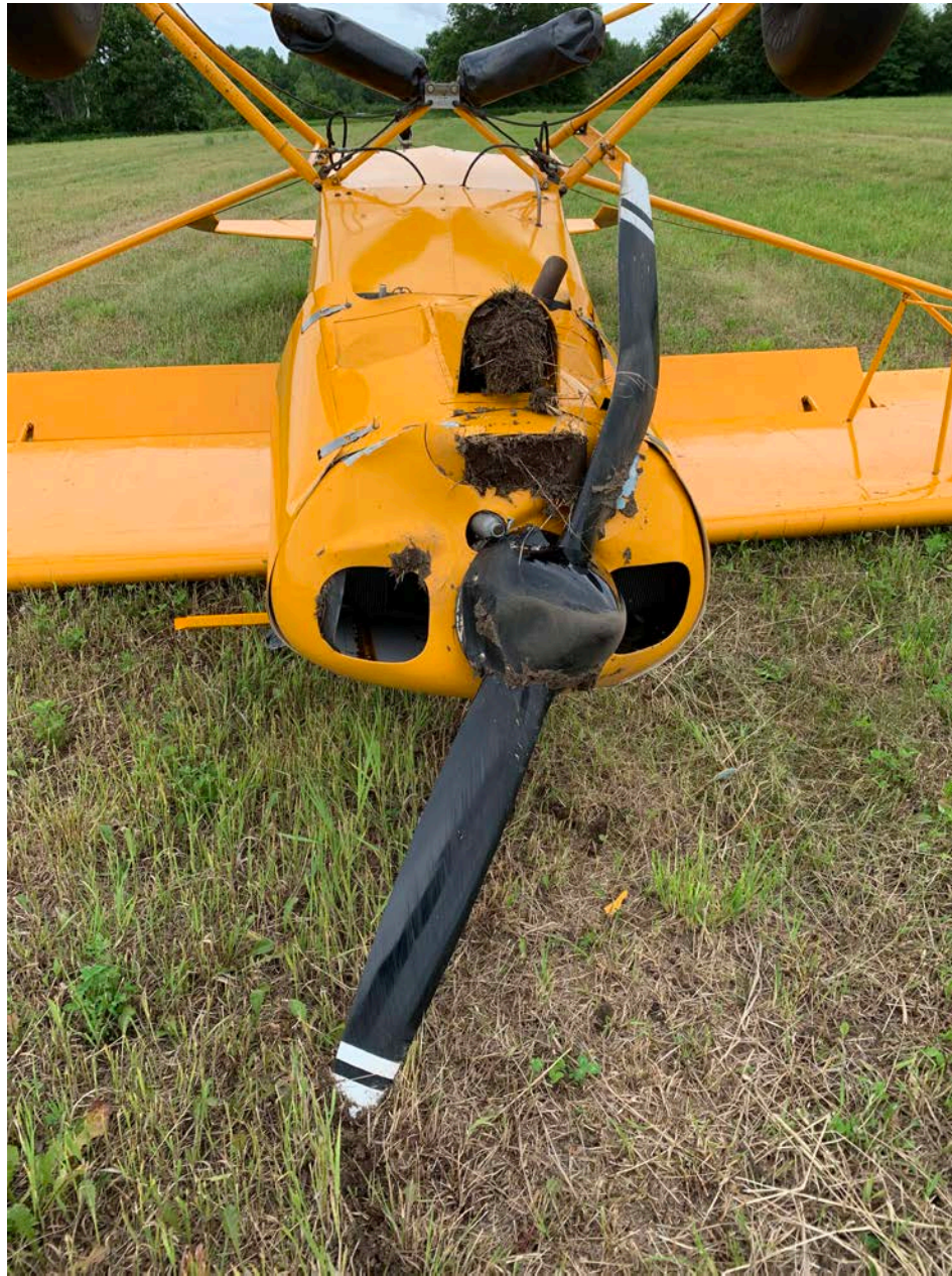
Photo 4 – Frontal damage to N7684D (FAA photo)
