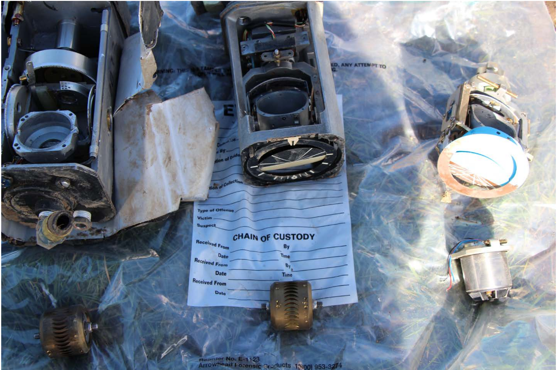
Photo 5 –Vacuum Driven Instruments Recovered from Accident Site
