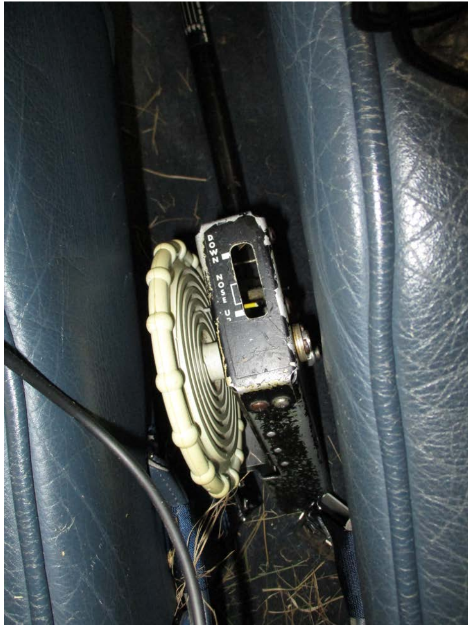
Photo 4 – View of the trim setting found after the accident (courtesy of the Federal Aviation Administration).
