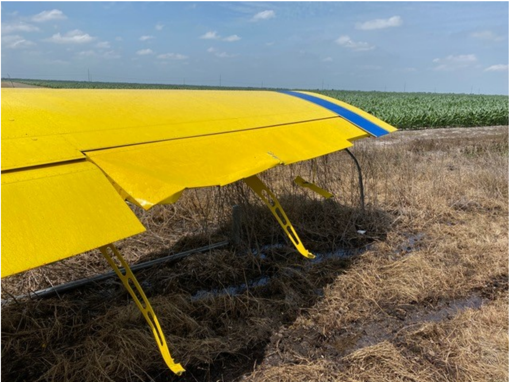
Photo 7 – View of the damaged right aileron (courtesy of Lane Aviation, Inc.).
