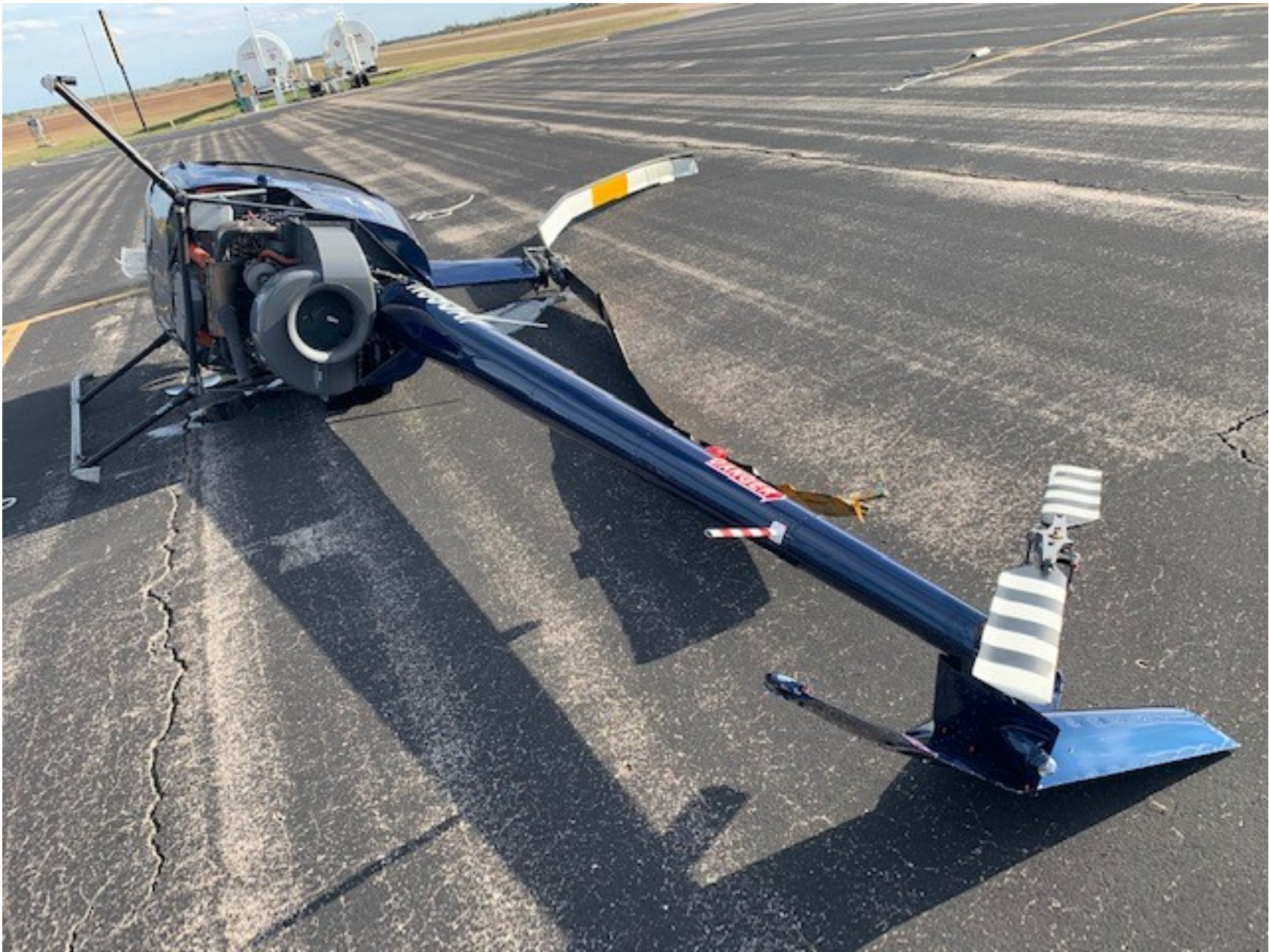
Photo 3 – View of the rear of the helicopter (courtesy of the certificated flight instructor).
