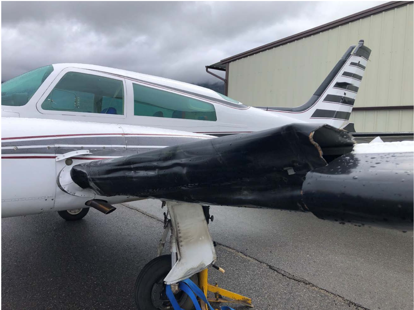
Photo – View of airplane with damage to the left wing (Courtesy of the FAA)
