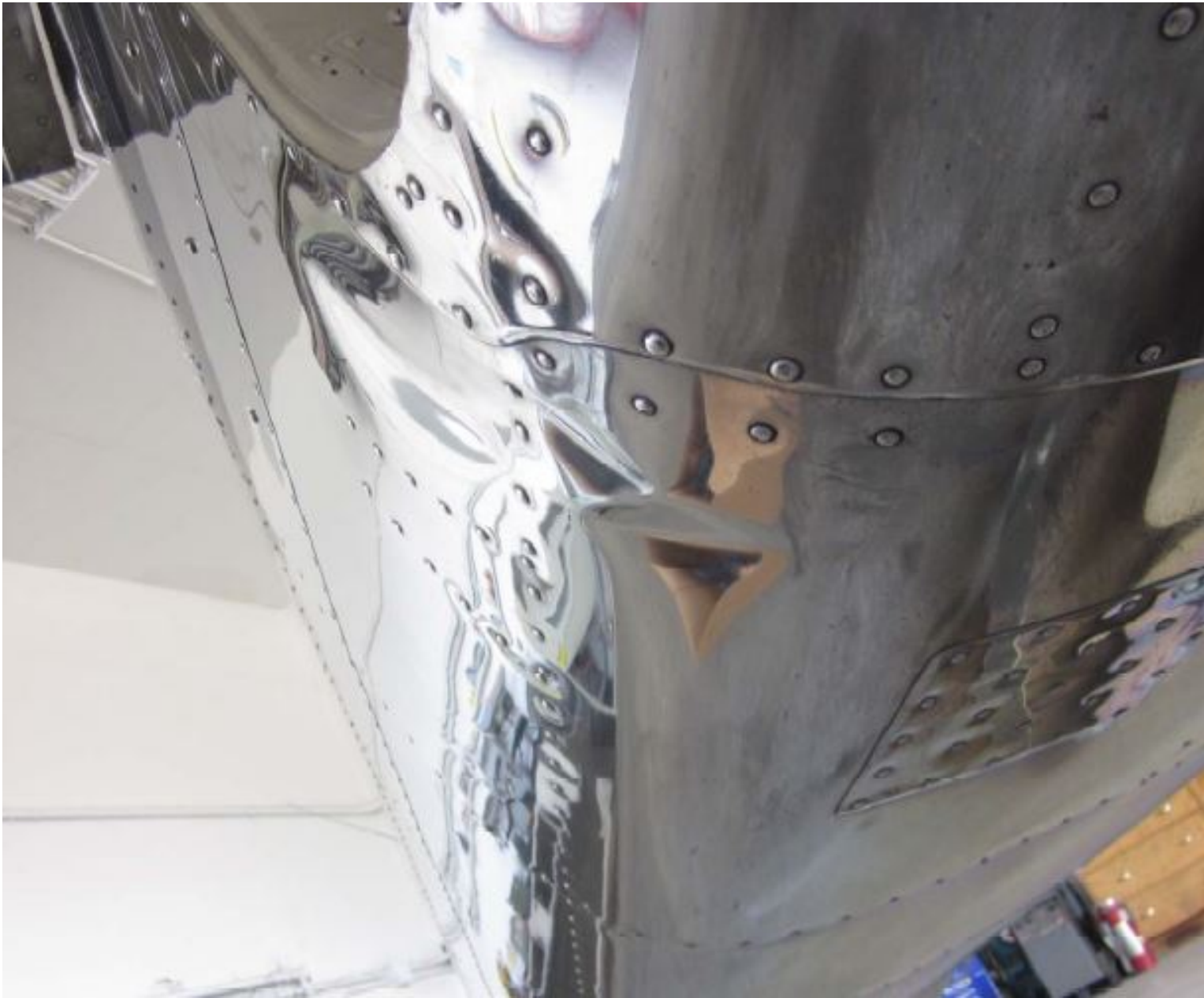
Photo 1 – View of damaged fuselage (courtesy of the FAA)
