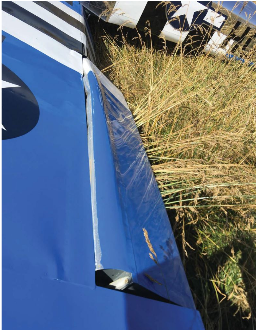
Photo – View of damaged left aileron (courtesy of the FAA)
