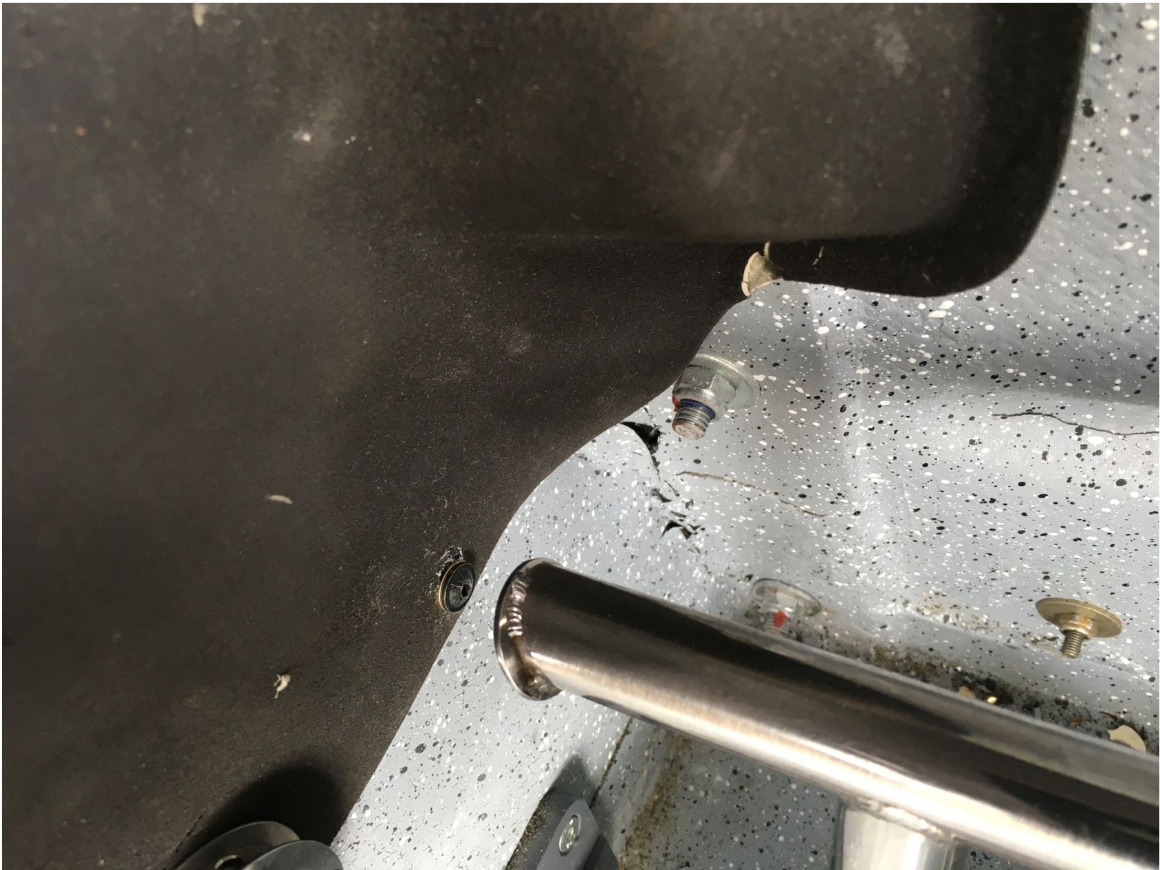
Photo 1 – View of damaged firewall forward of rudder pedals (courtesy of the FAA)
