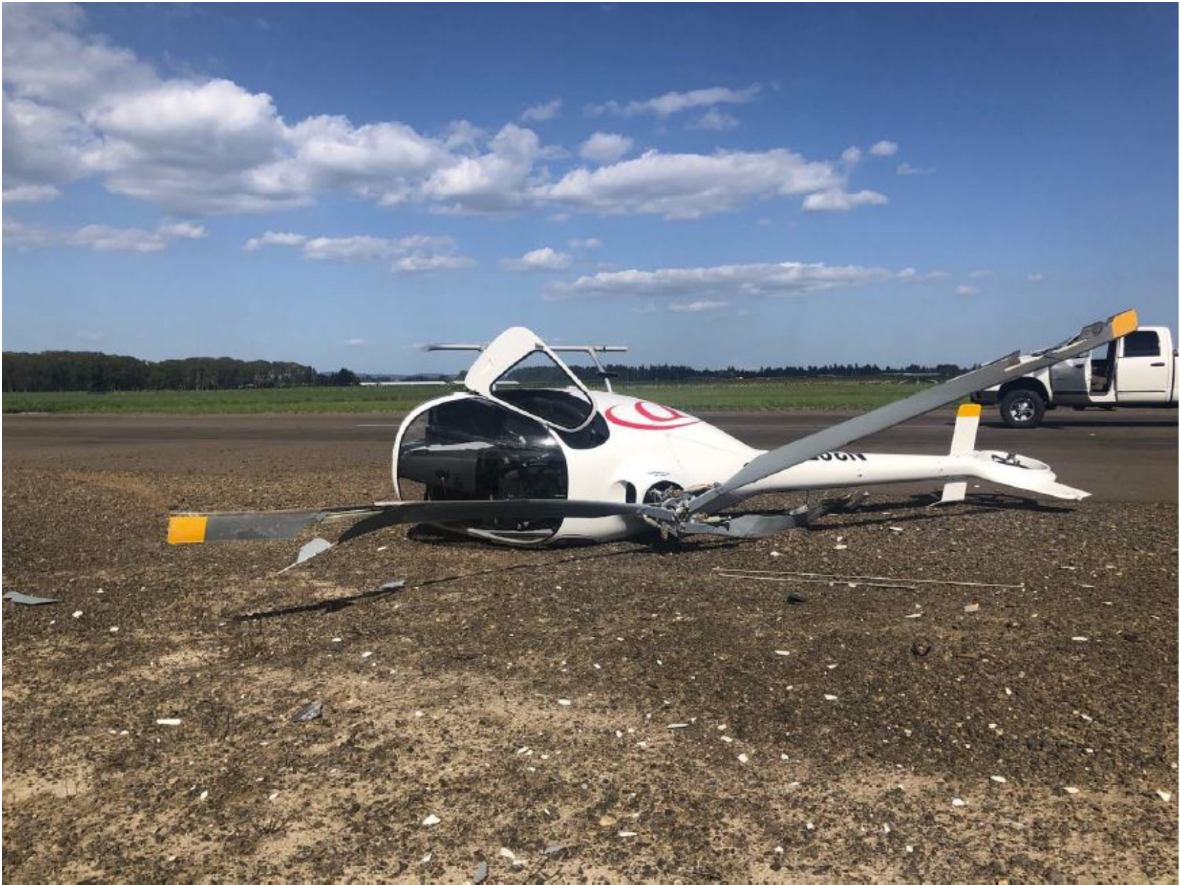
Photo 1 – View of helicopter resting on its left side with damage to main rotor blades (courtesy of the FAA)
