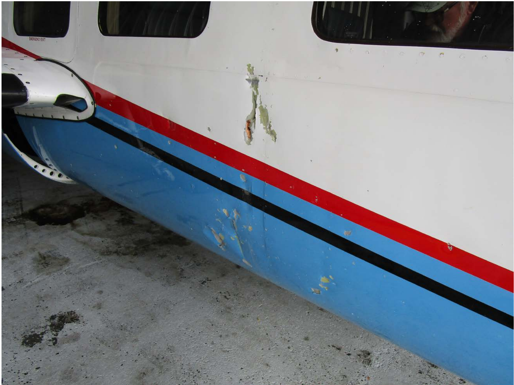
Photo 1 – View of damaged pressurized cabin (courtesy of the FAA)
