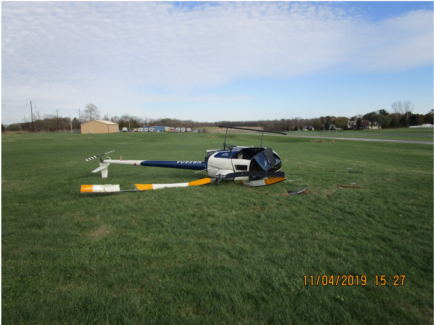
Photo 1 – View of damaged main rotor blades and horizontal stabilizer (courtesy of the FAA)
