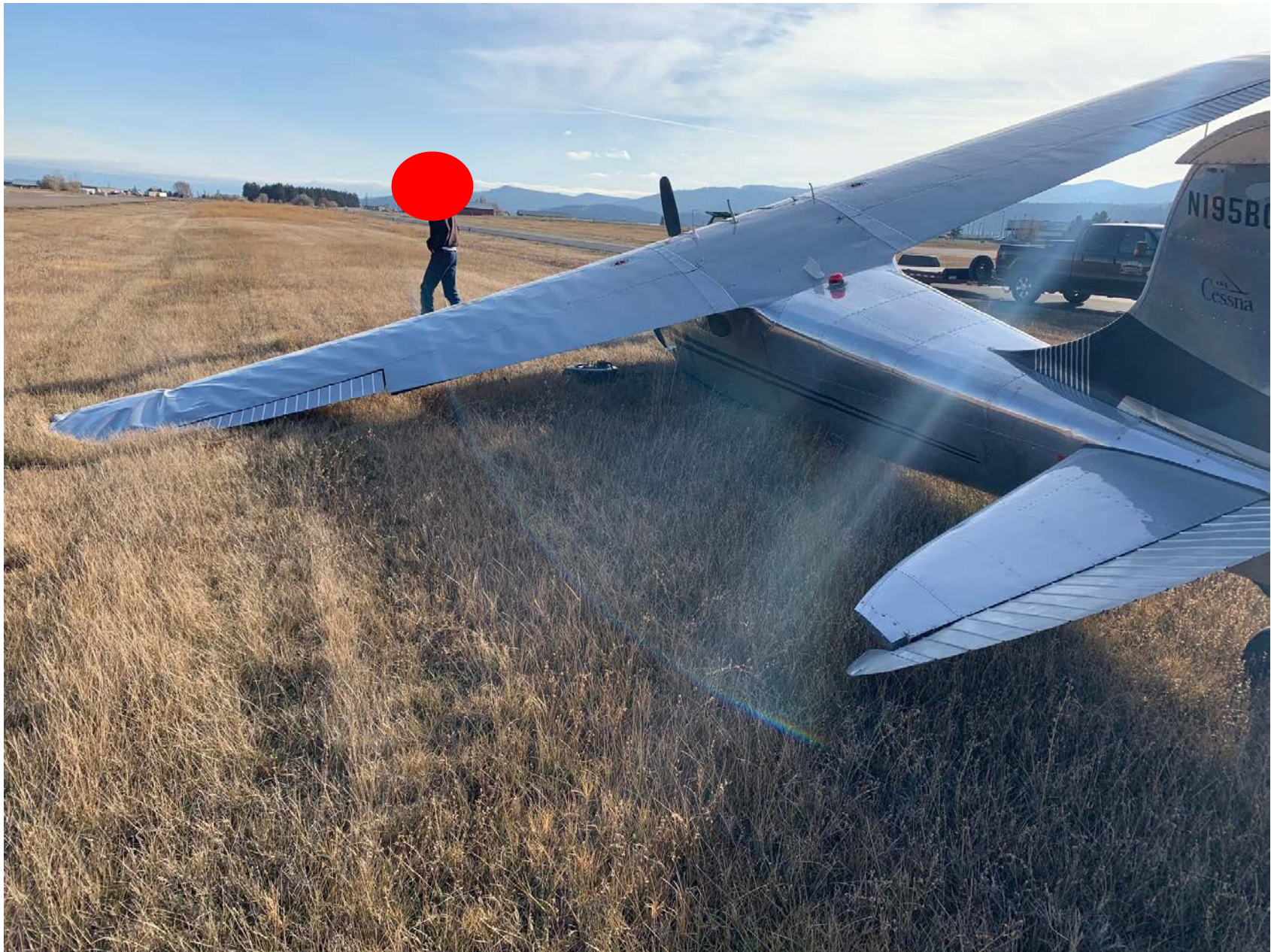
Photo 1 – View of damaged left wing (courtesy of the FAA)
