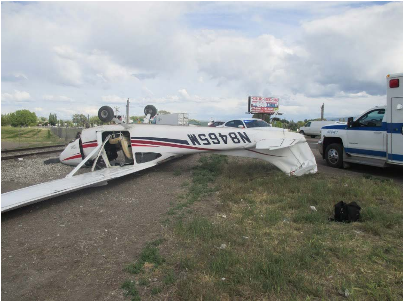
Photo 1 – View of damaged empennage and right-wing lift strut (courtesy of the FAA)
