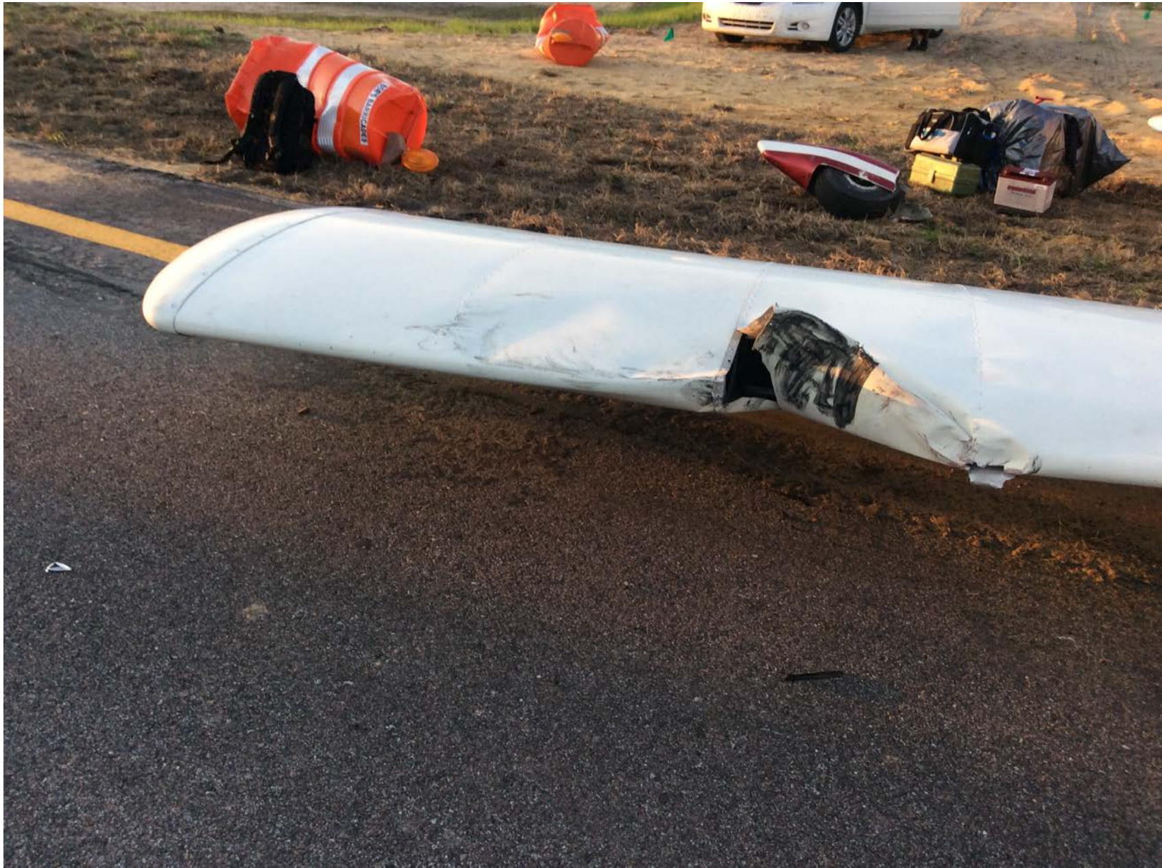
Photo 1 – View of damaged right wing (courtesy of the FAA)
