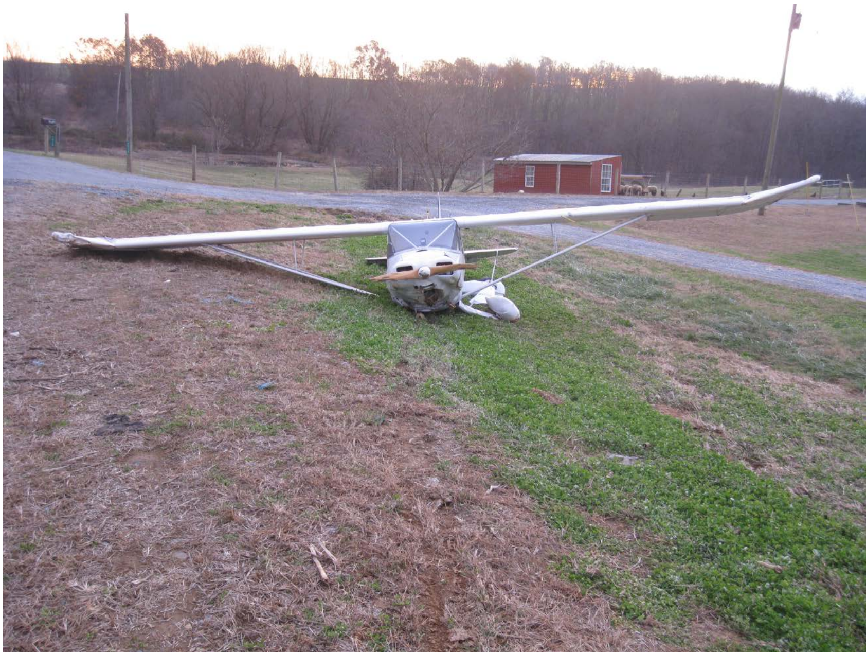
Photo 1 – View of damage to both wings (photo courtesy of the Pilot)
