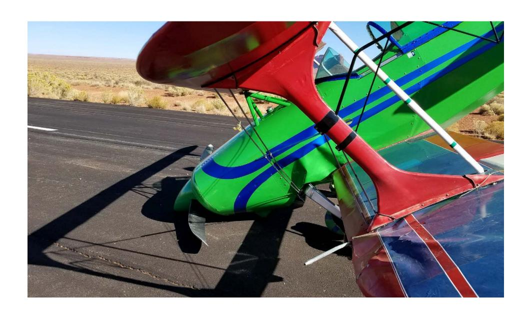
Photo 1 – View of fuselage and lower left wing damage (photo courtesy of unknown)
