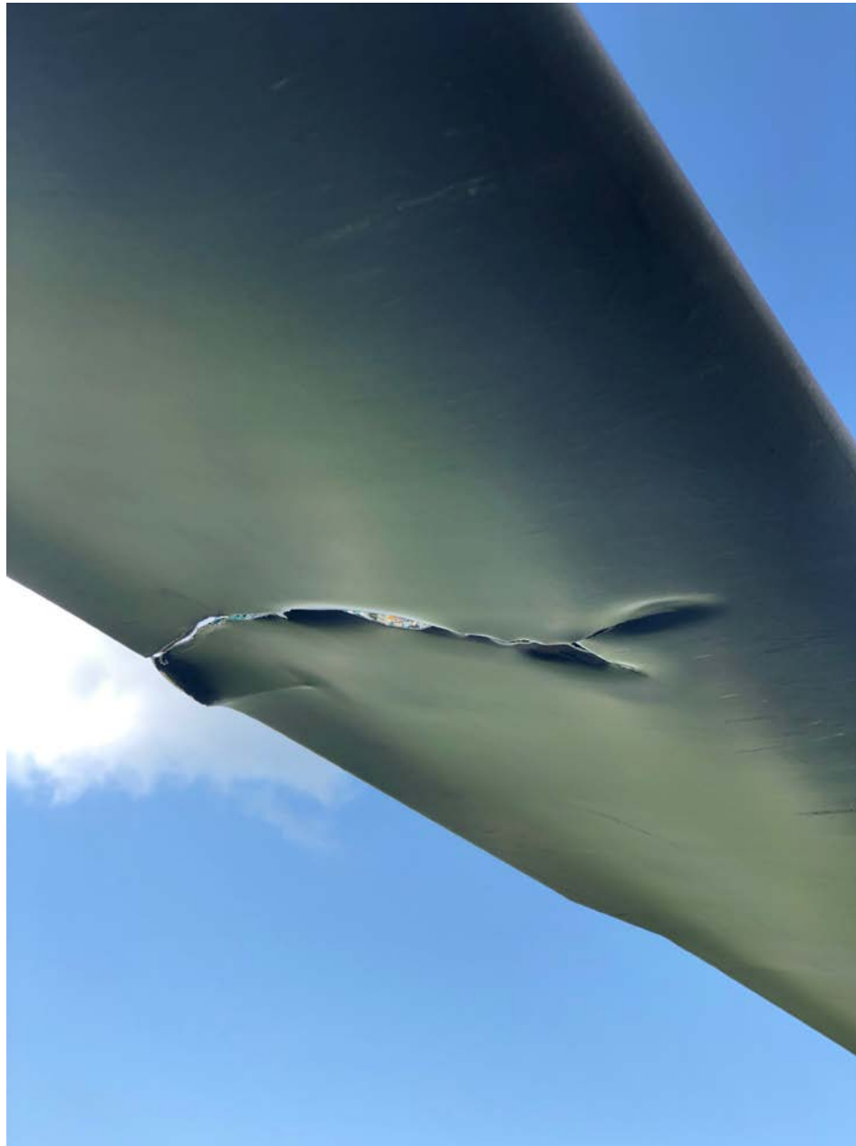
Photo 1 – View of damaged main rotor blade (courtesy of the pilot)
