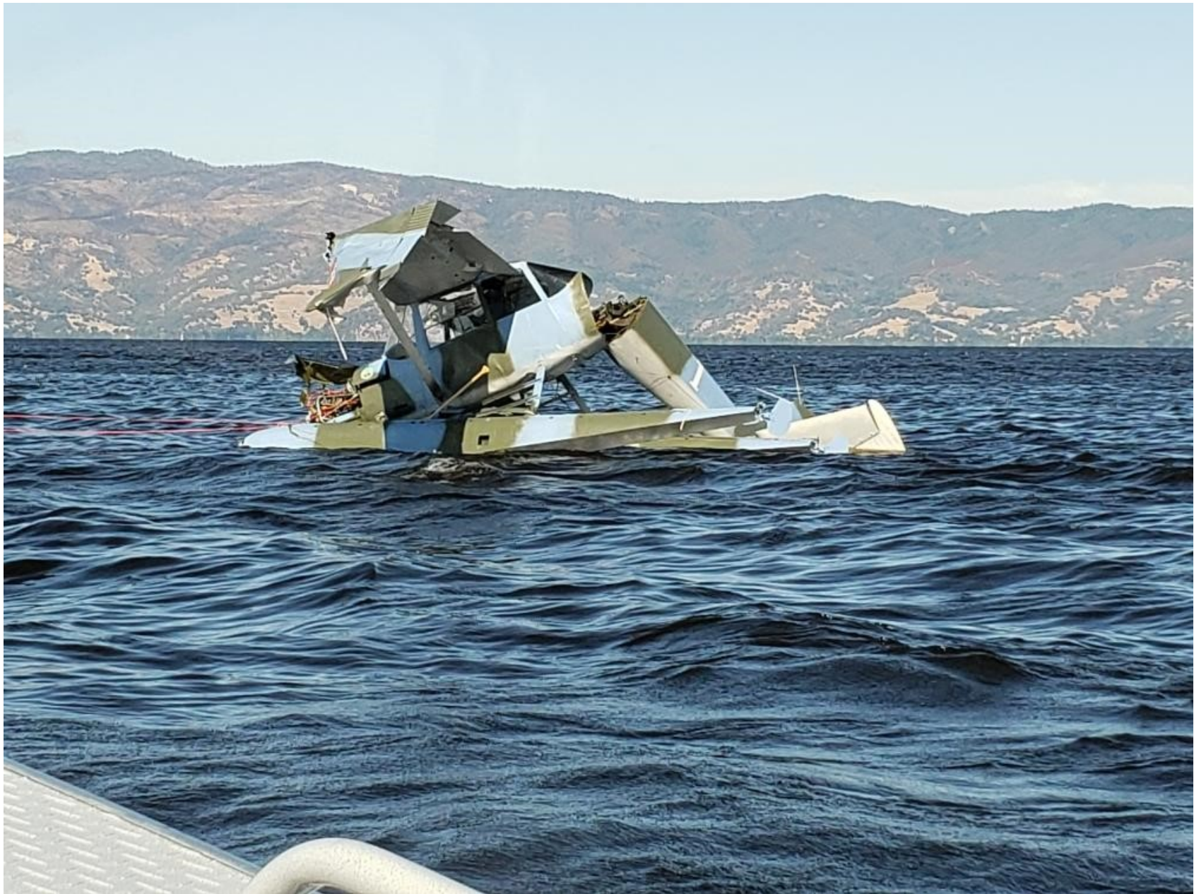
Photo 1 – View of fuselage and left wing damage (photo courtesy of local law enforcement).
