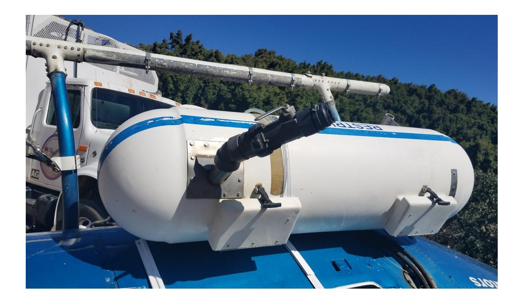
Photo 2 – View of loading hose attached to aerial application tank (courtesy of the FAA)
