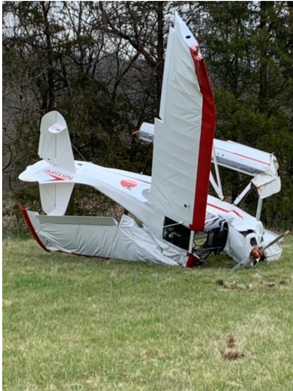
Photo 1 – View of damage to both wings (courtesy of the FAA)
