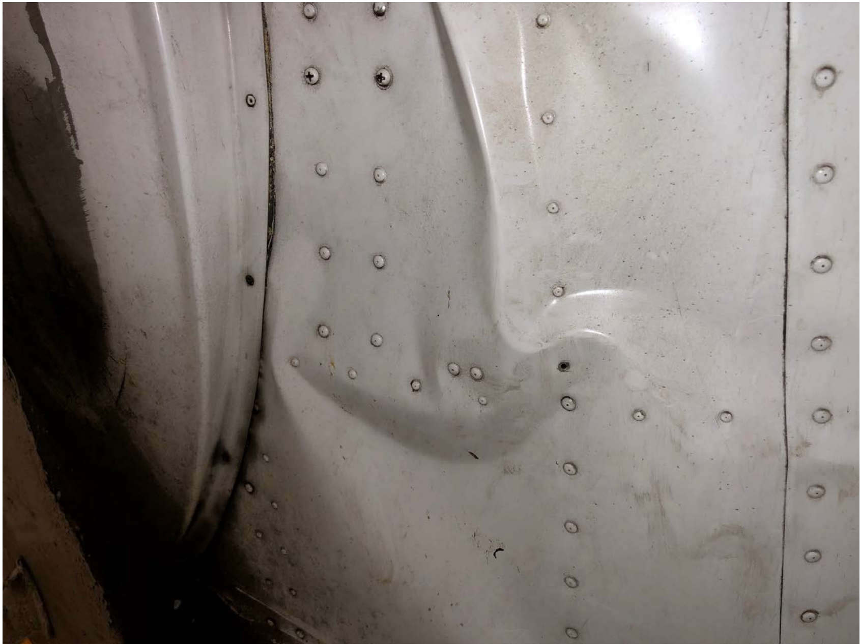
Photo 1 – View of bottom fuselage damage (photo courtesy of the FAA)
