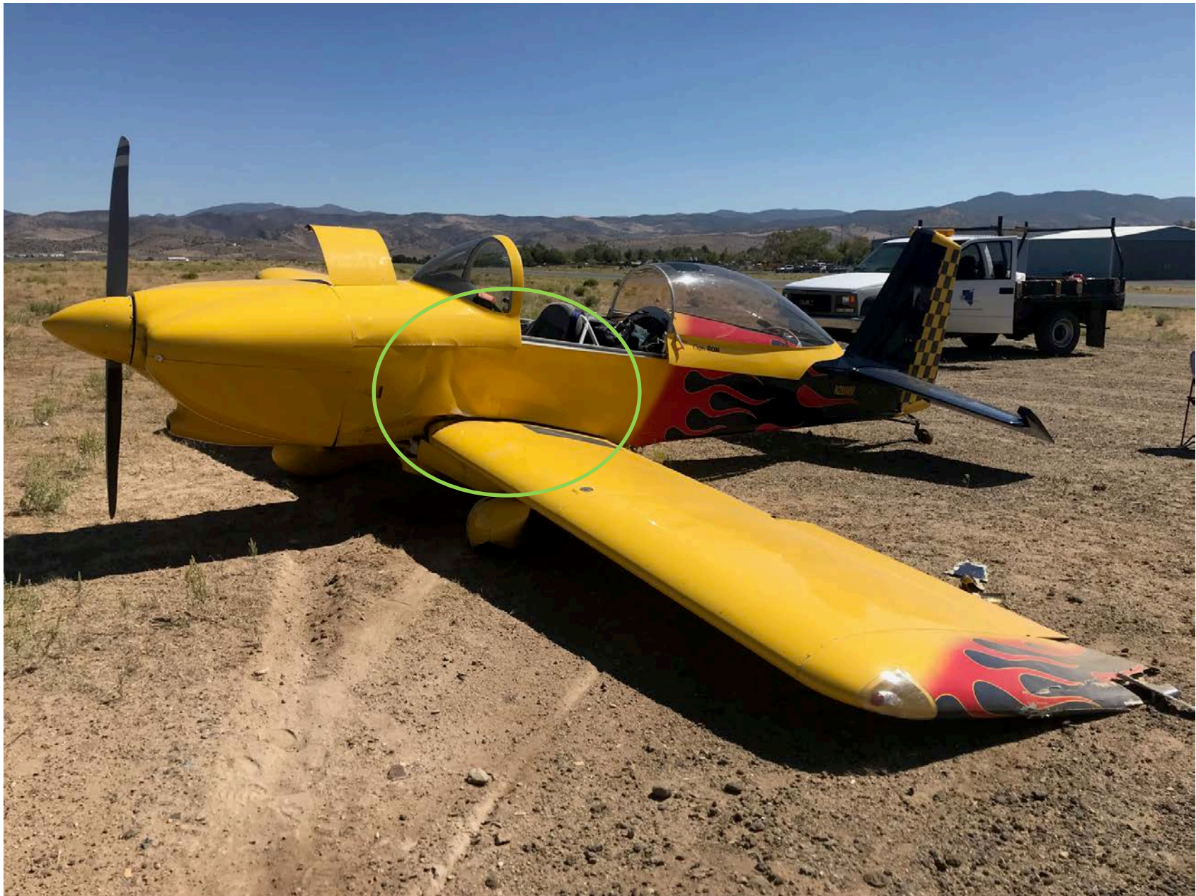
Photo – View of damage to fuselage (photo courtesy of the FAA)
