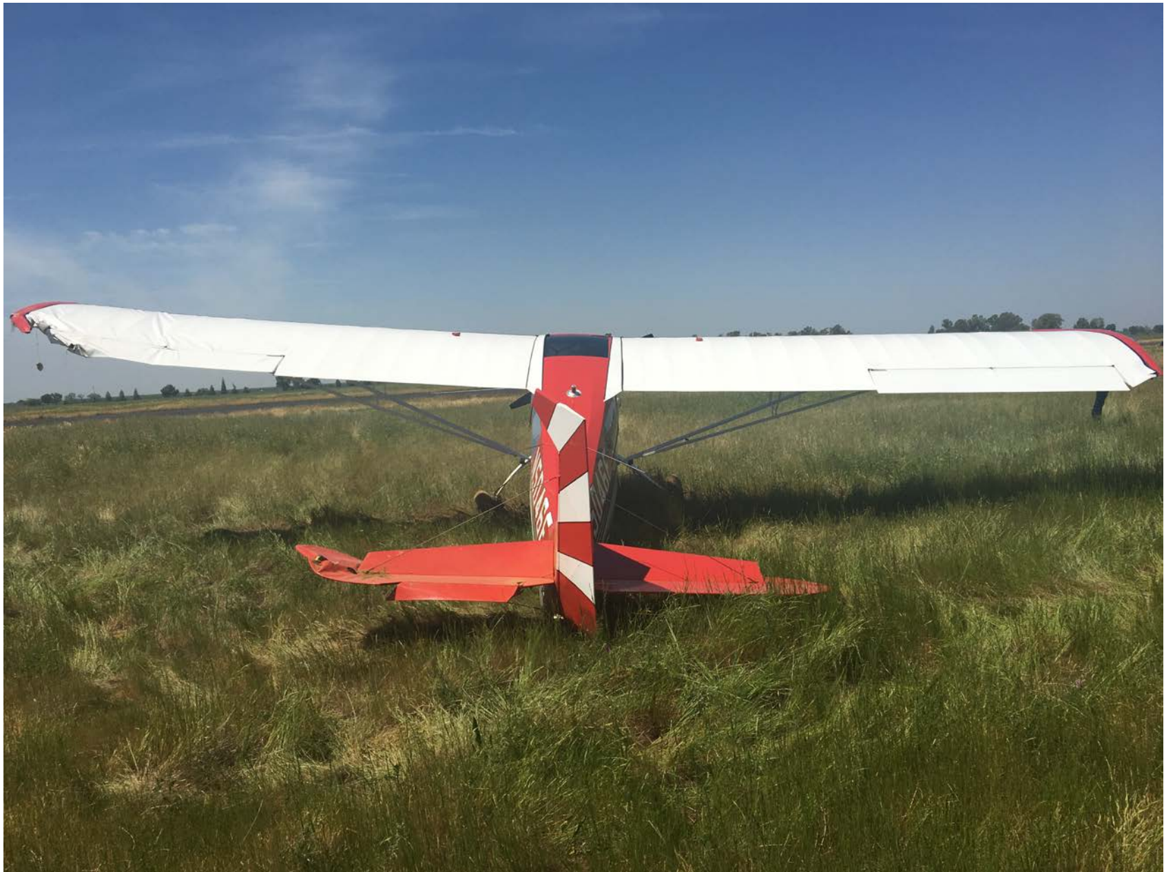
Photo 1 – View of left wing and left elevator damage (photo courtesy of the FAA)
