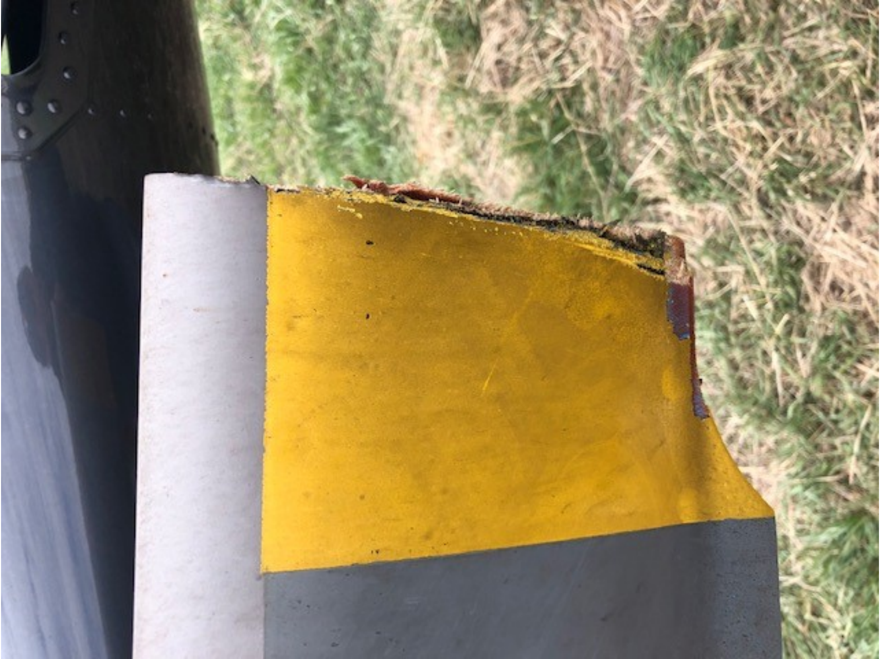
Photo 1 – View of damaged tail rotor blade (Photo courtesy of the operator)
