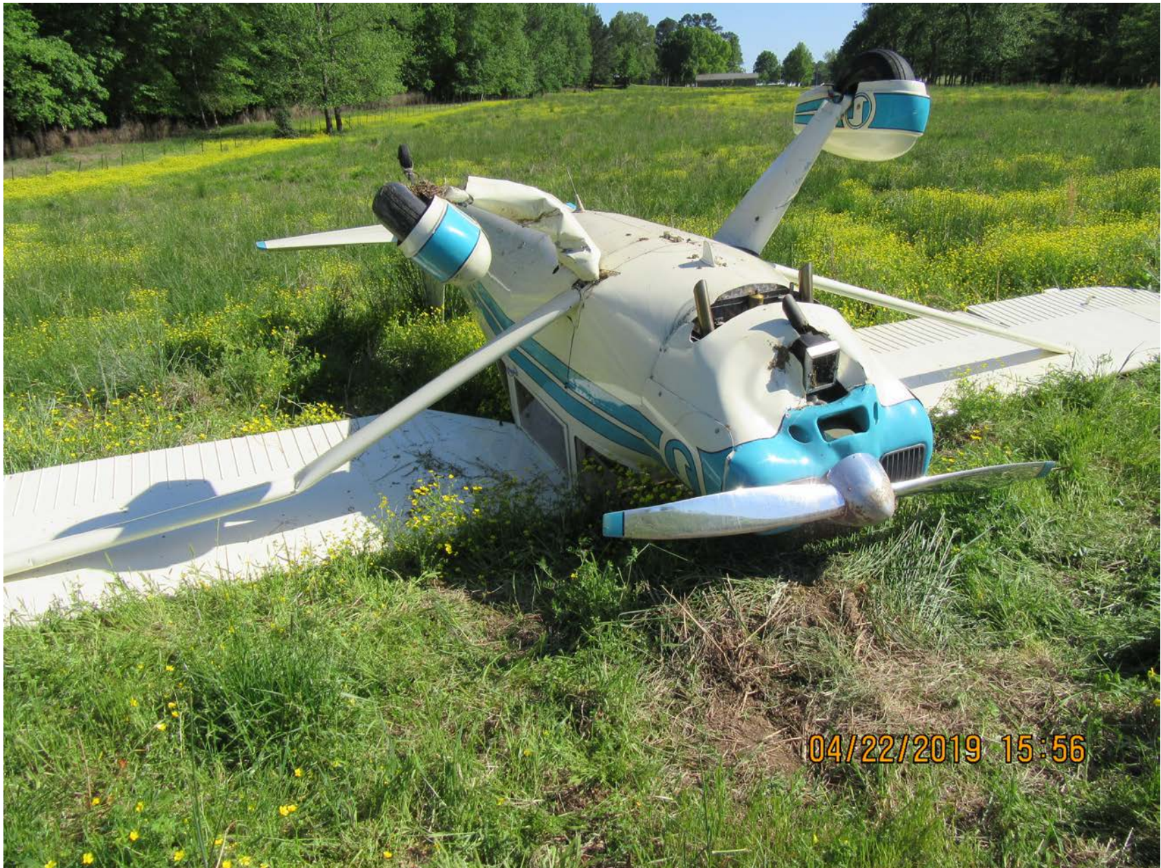
Photo 1 – View of left wing and wing strut damage (photo courtesy of the Pilot)
