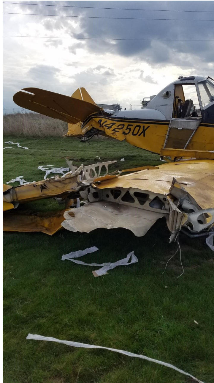
Photo 1 – View of damaged right wing and empennage (Photo courtesy of the pilot)
