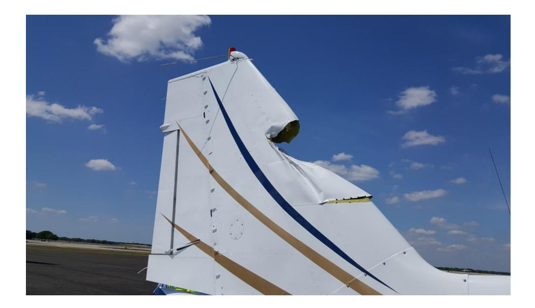
Photo 1 – View of vertical stabilizer damage (photo courtesy of the FAA)
