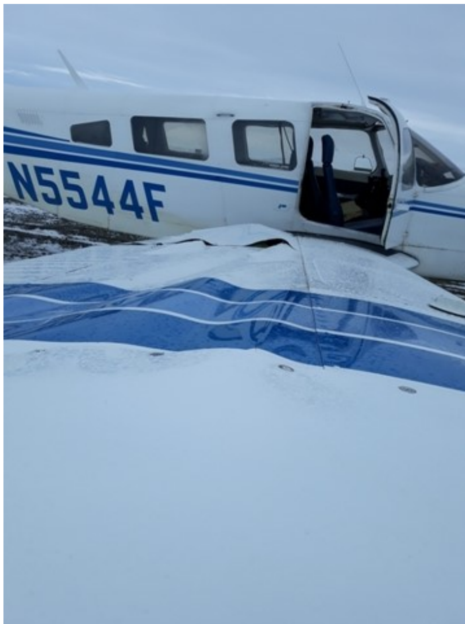
Photo 1 – View of right wing damage (photo courtesy of the FAA)
