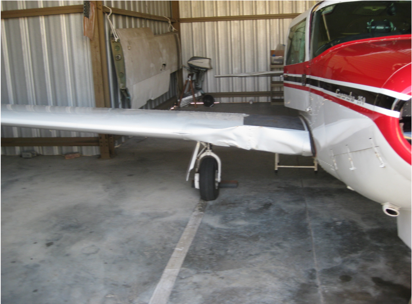
Photo 1 – View of damaged right wing and right horizontal stabilator (Photo courtesy of the FAA)
