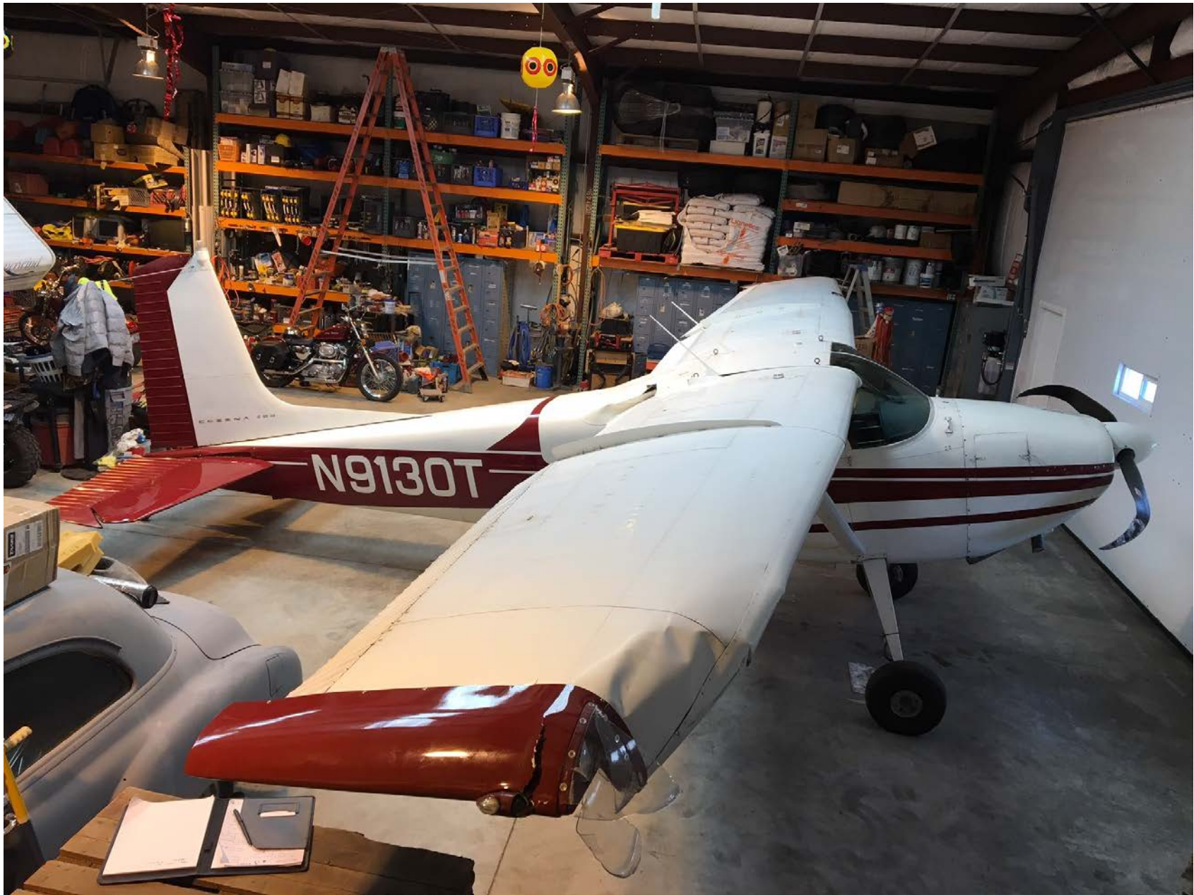
Photo 1 – View of damaged right wing
