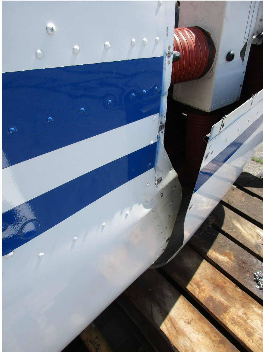
Photo 1 – View of damaged fuselage (Photo courtesy of the FAA)
