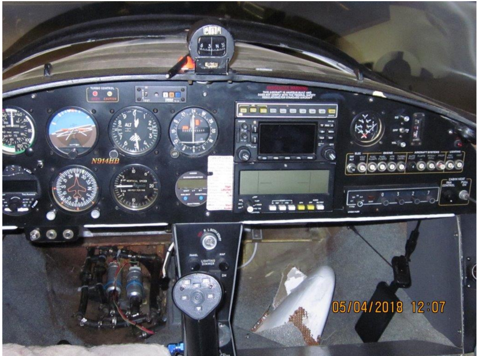
Photo 1 – View of damaged floorboard (Photo courtesy unknown)
