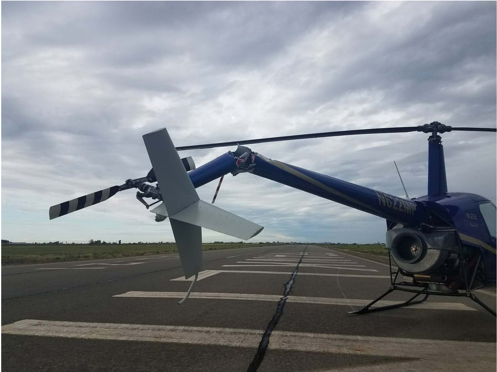
Photo 1 – View of damaged tailboom (Photo courtesy of the Chief Pilot)
