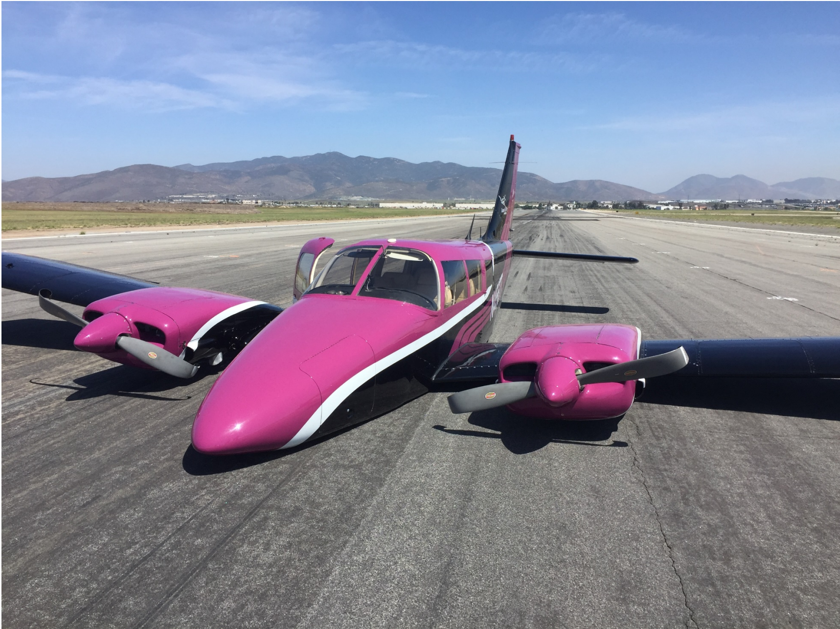
Photo 1 – View of airplane after landing with the gear retracted (Photo courtesy of the FAA)
