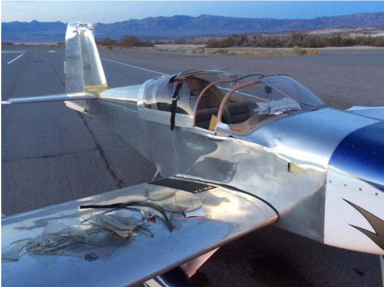
Photo 1 – View of damaged canopy and empennage (Photo courtesy unknown)
