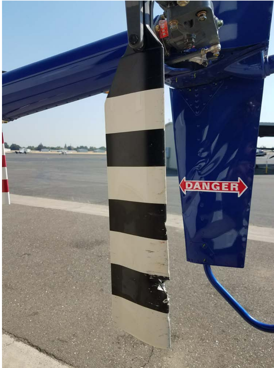
Photo 1 – View of damaged vertical stabilizer (photo courtesy of the General Manager of the flight school)
