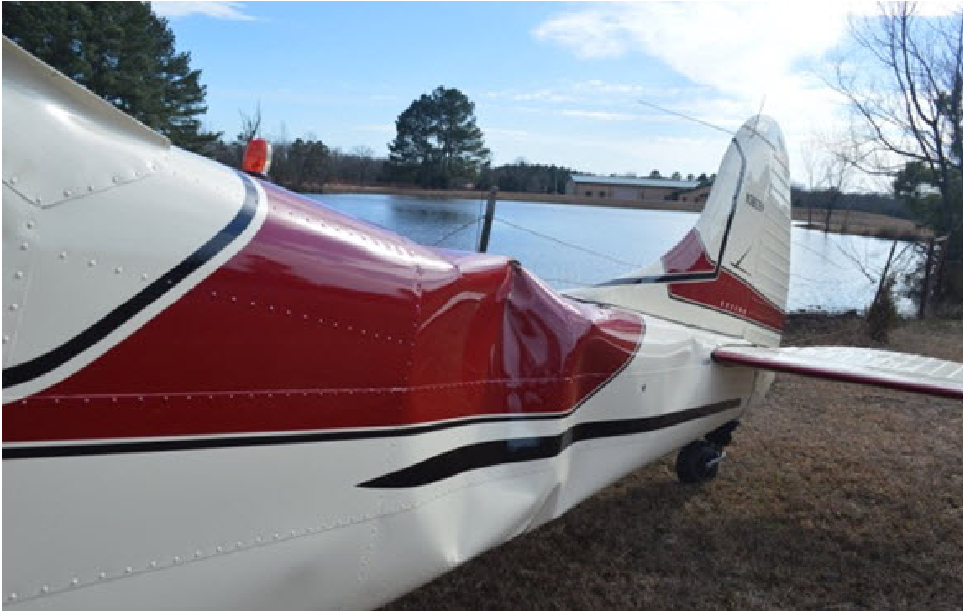
Photo 1 – View of fuselage damage (photo courtesy of the pilot)
