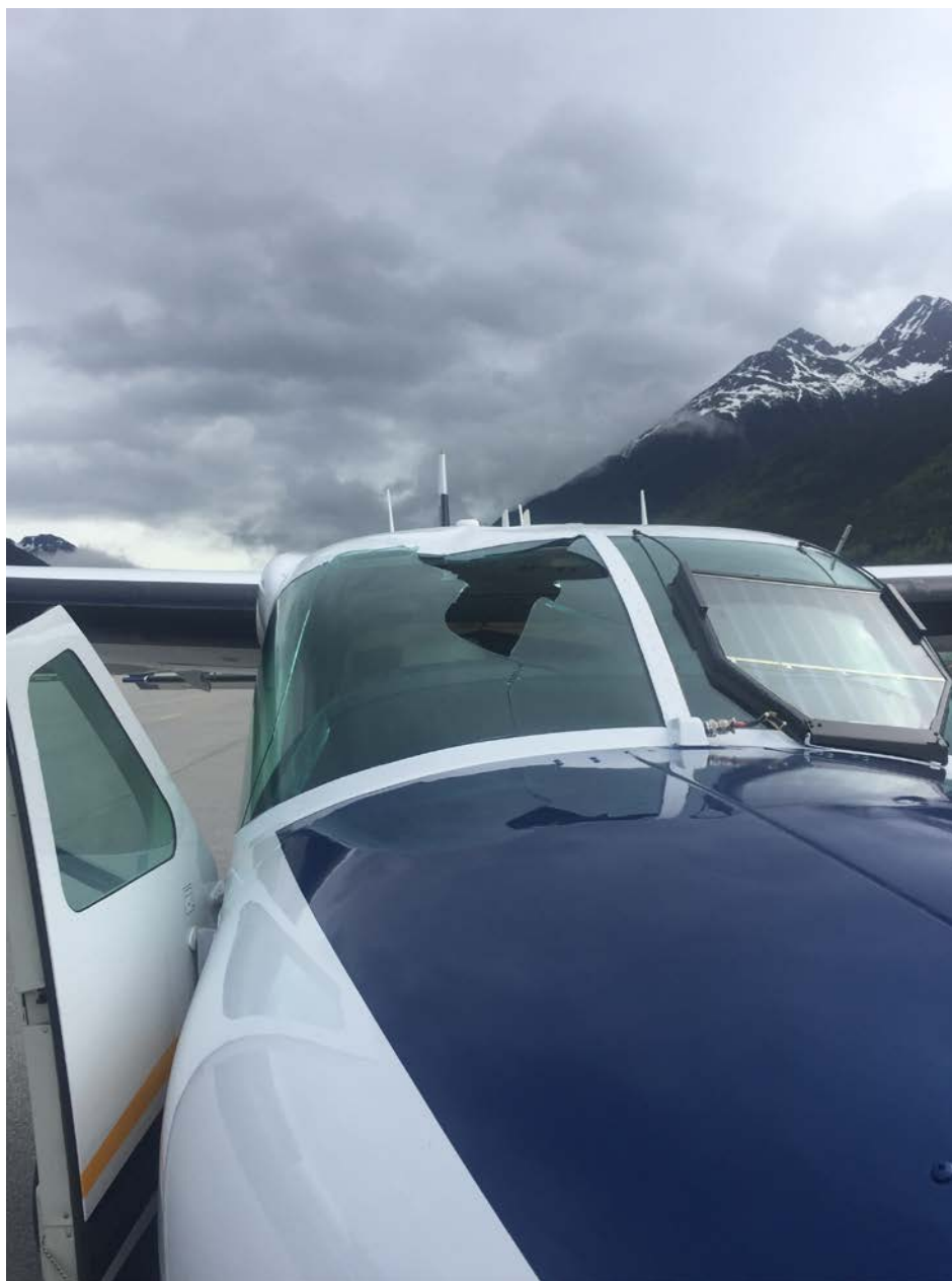
Photo 1 – View of damaged windscreen and fuselage (photo courtesy of the operator)
