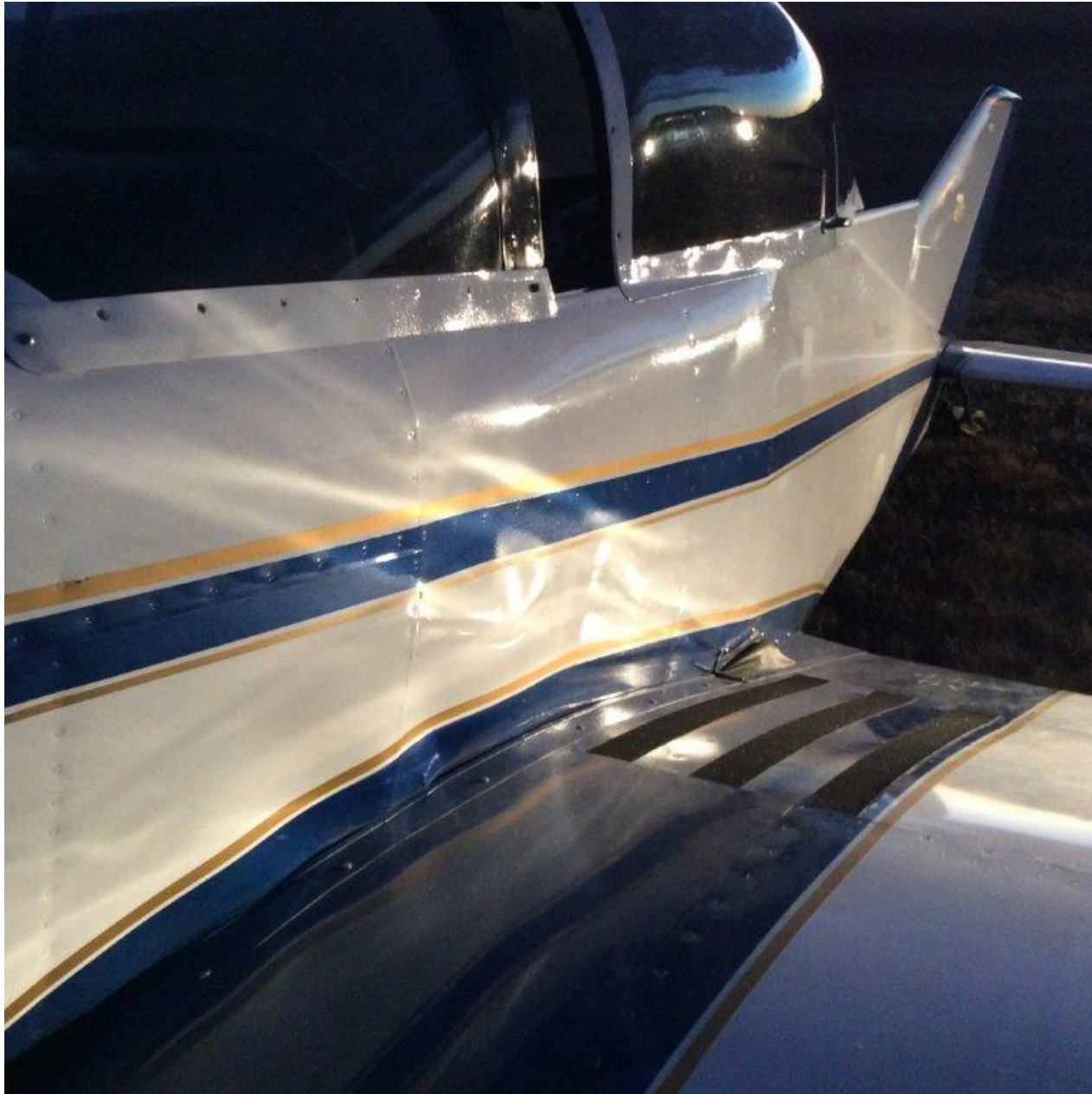
Photo 1 – View of damaged fuselage (photo courtesy of the FAA)
