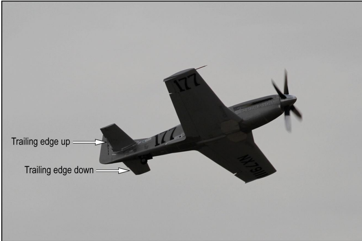
Figure 8. Airplane pitching up with left elevator trim tab trailing edge down at 1624:30.34, right elevator trim tab trailing edge up, and nearly full right-wing-down aileron deflection.
