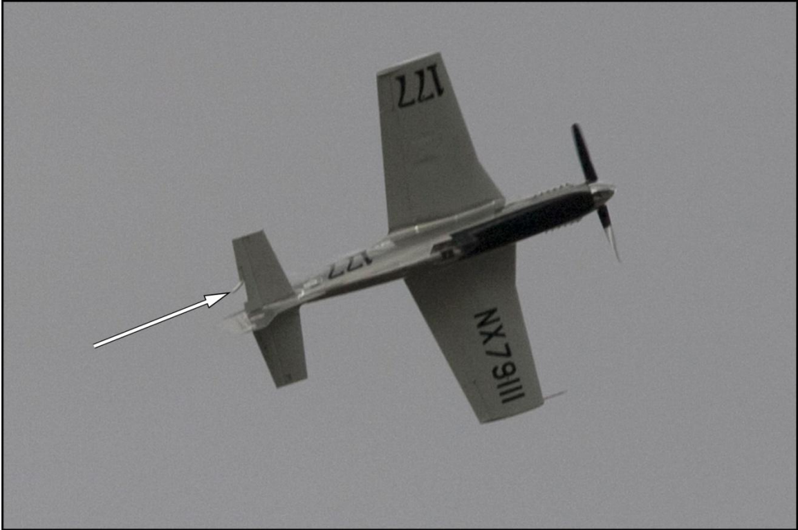
Figure 9. Inboard piece of left elevator trim tab detached from inboard hinge.
