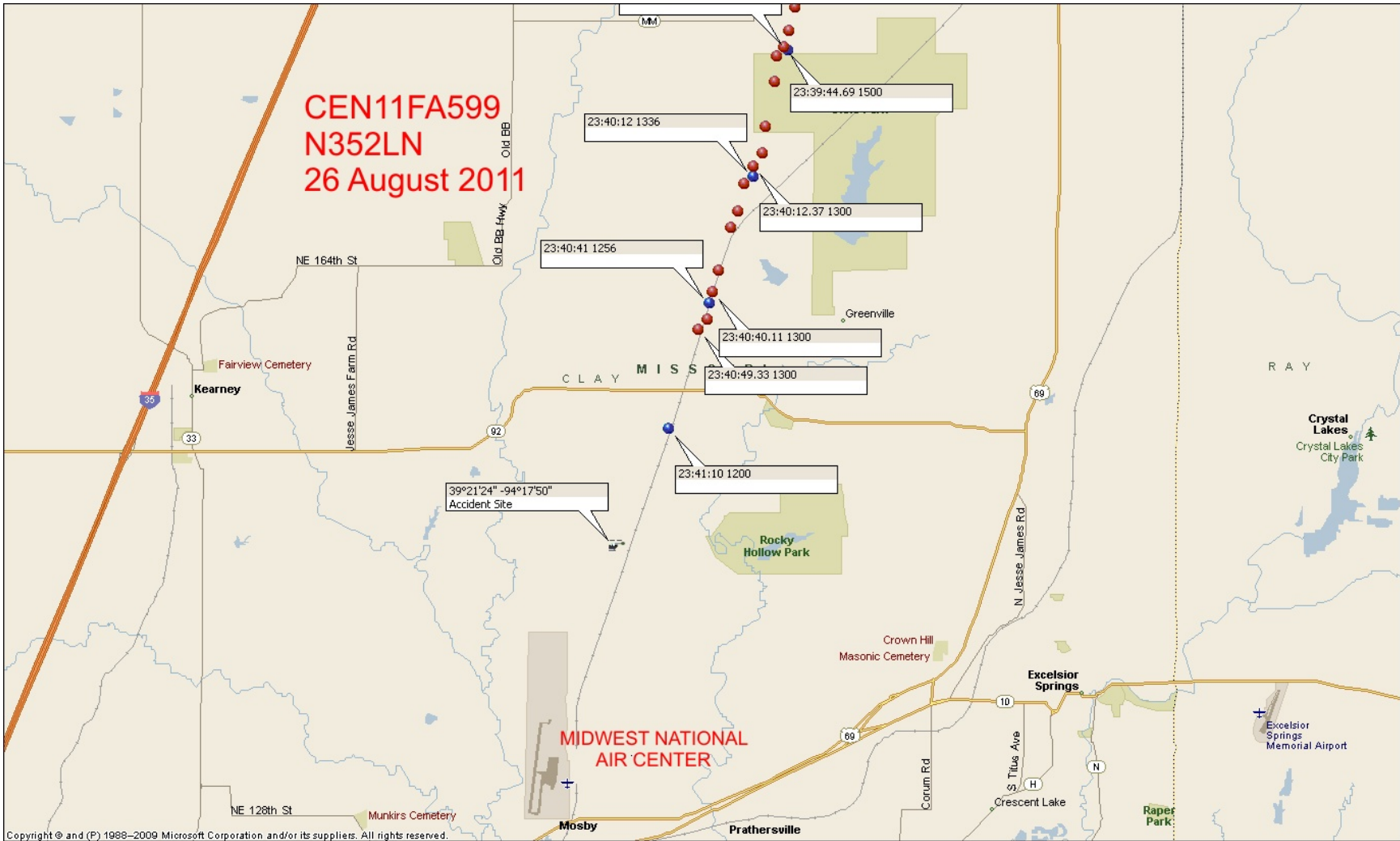
Figure 5 – Last radar targets and GPS position reports, along with the location of the destination airport.
