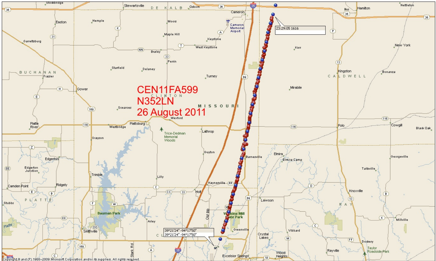
Figure 2 – KCI radar data (red dots) and Air Methods tracking data (blue dots) from 2329Z until the end of the flight.
