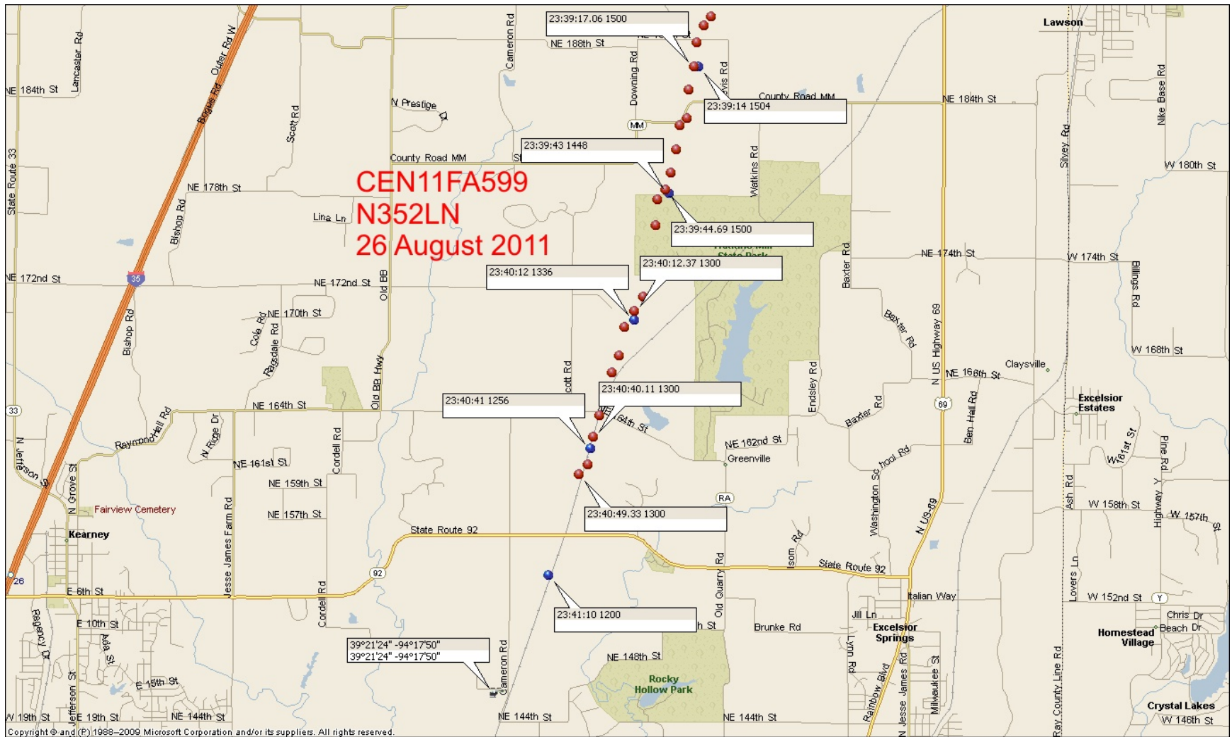
Figure 3 – KCI radar data (red dots) and Air Methods tracking data (blue dots) for approximately the last two minutes of the flight. Tags show mode C altitude reports from KCI and GPS-derived altitude from Air Methods.
