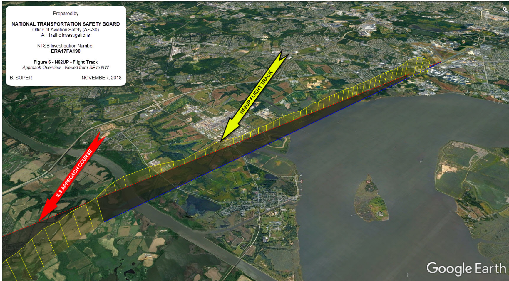
Figure 6 - Radar flight track of the final segment of the accident flight of N62UP. This figure is an overhead view of the flight track looking from southeast to northwest with the ILS approach course also depicted to illustrate an overview of the approach.
