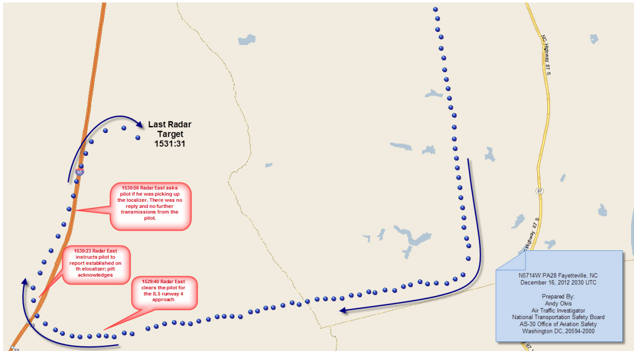
Figure 6 - Radar track of N5714W being vectored back to FAY.
