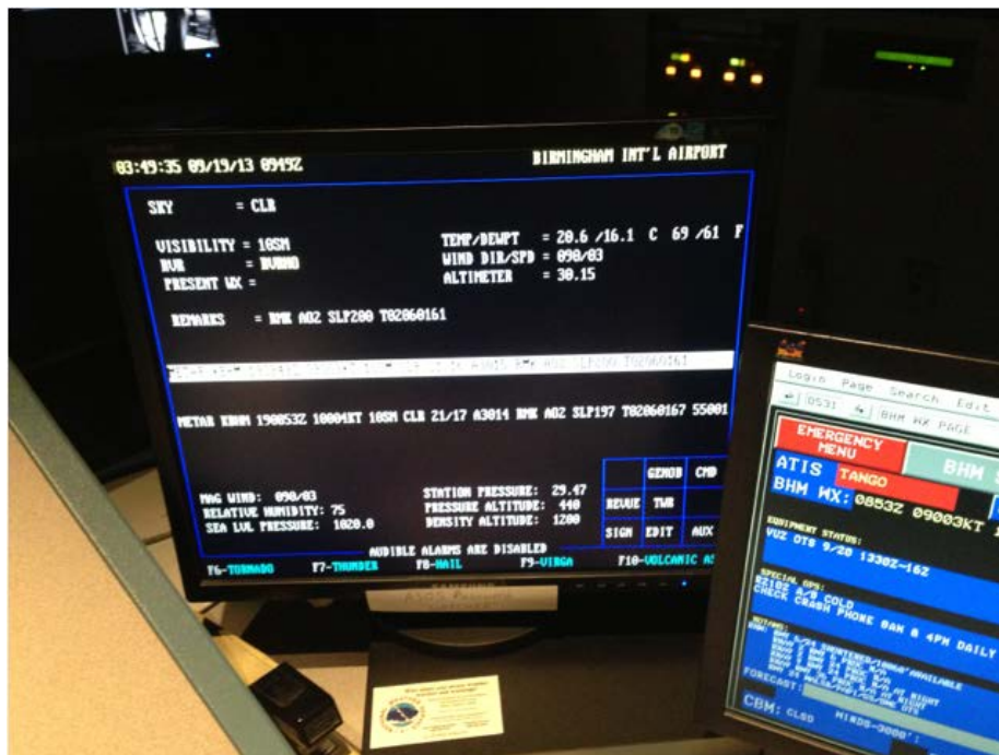
Figure 5 – BHM ASOS Monitor located in the BHM ATCT
