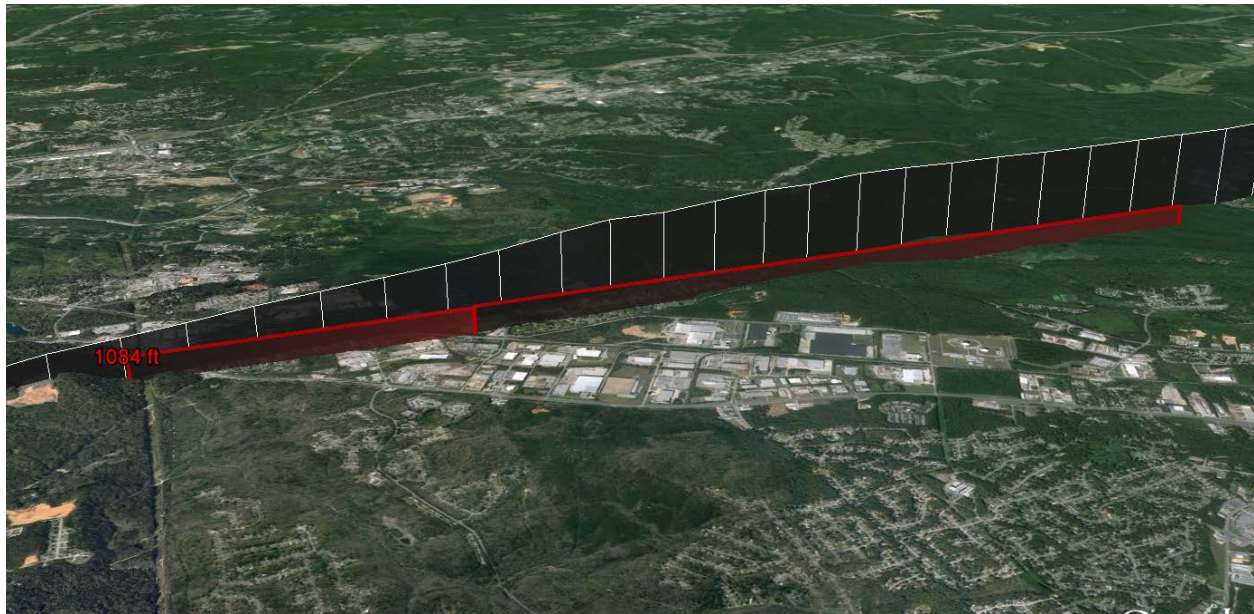
Figure 9 – The UPS1354 radar flight path is indicated by the white line and the 2 segment MSAW type II area current initiate monitor altitude is indicated by a red line.
