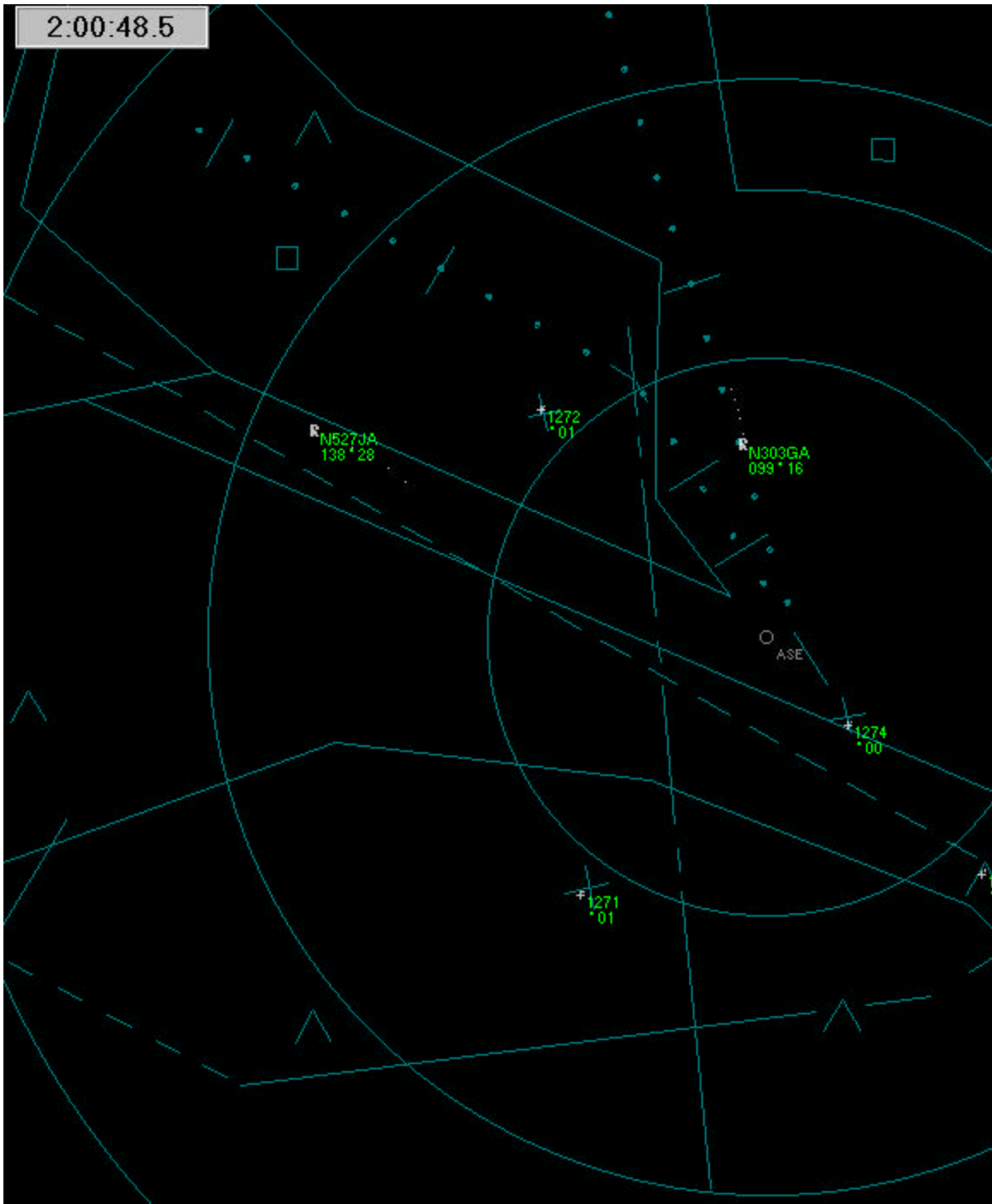
Overlay of ASE Radar Tracking Data on simulation of D-BRITE Video Map
