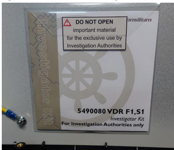
Figure 6. Consilium VDR investigator kit, secured inside the main unit
