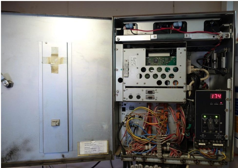
Figure 3. Furuno VDR main unit, interior
