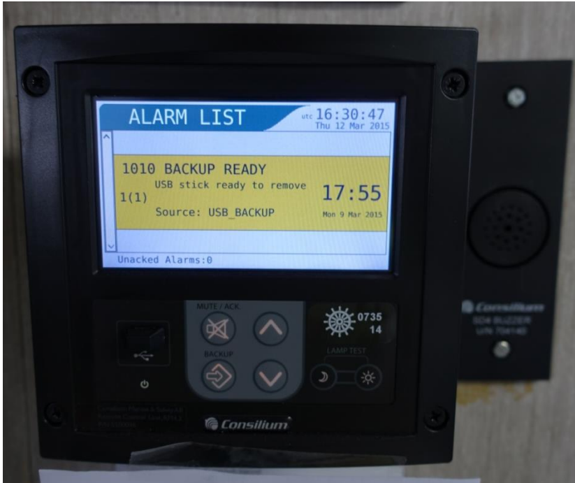
Figure 4. Consilium VDR remote control unit, as investigators arrived onboard (March 12, 2015)
