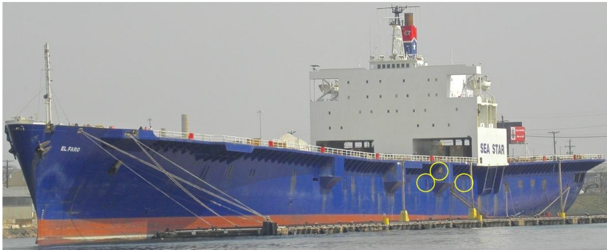
Figure 6-8: EL FARO port side showing ventilation supply and exhaust louvered hull openings. The openings for Hold 3 are highlighted. Photo copyright Will Van Dorp, used with permission.
