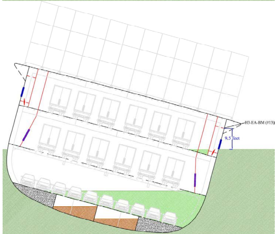
Figure 6-18: Scaled drawing of sections at frame 143 (Hold 3 ventilation supply trunk) and frame 159 (Hold 3 aft ventilation exhaust trunk), with flooding of Hold 3 to 20% with permeability 0.7 and heel angle of 15 degrees shown for example.
