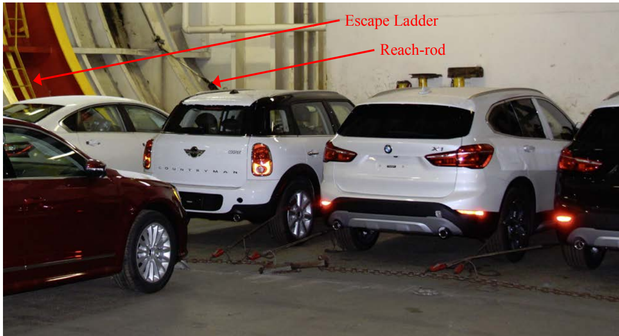
1 2 Figure 14. Cars lashed on El Yunque during loading in hold 3, tanktop, looking aft and to port. 3 Escape ladder and emergency fire pump reach-rod in left background. (Photo from December 4 2015)
