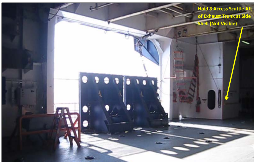
1 2 Figure 13. El Faro starboard sideshell opening with installed bulwark. (Screen capture from video 3 by former El Faro second mate, September 2008 256 )
