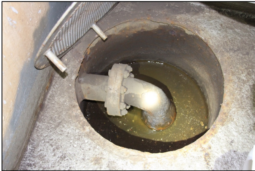
5 Figure 21. El Yunque hold 3 tanktop, portside bilge drainwell (rosebox) with cover screen lifted. 6 (Photo from December 2015)
