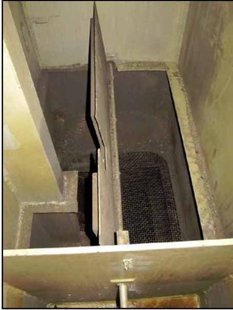
1 2 Figure 33. El Yunque , cargo hold 3, exhaust trunk fire damper at frame 161.5. Left image is top 3 view of damper, right image is a side view looking outboard. (Photo from September 2016)
