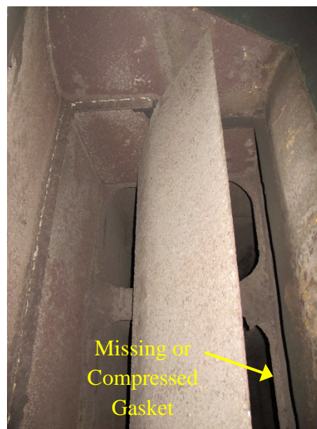
4 Figure 31. El Yunque , hold 2A starboard ventilation supply fan and fire damper housing on 5 second deck (left), internal fire damper/closing appliance (right). Damper's rubber gasket was 6 missing or compressed around most of seal perimeter. (Photo from September 2016)
