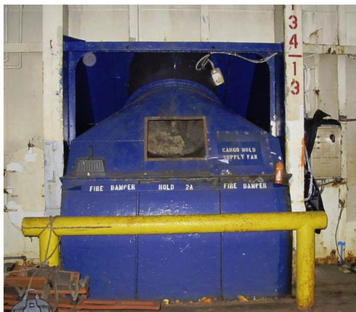
4 Figure 31. El Yunque , hold 2A starboard ventilation supply fan and fire damper housing on 5 second deck (left), internal fire damper/closing appliance (right). Damper's rubber gasket was 6 missing or compressed around most of seal perimeter. (Photo from September 2016)
