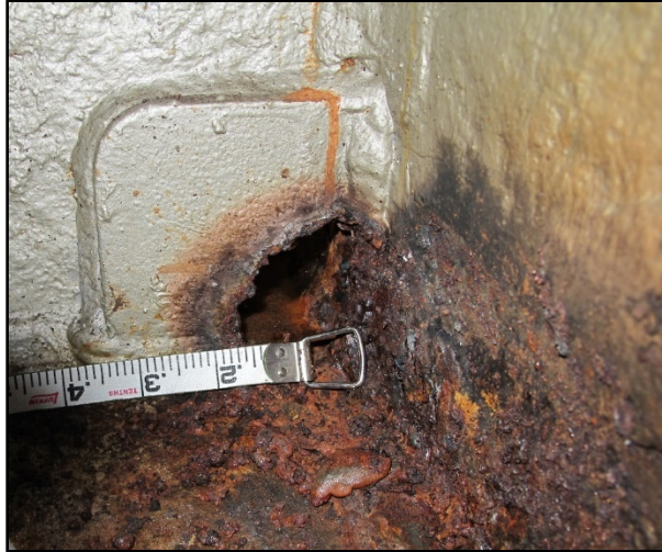
2 Figure 34. El Yunque , 1.5-inch-radius drainhole inside cargo hold 3 ventilation trunk, second deck 3 at frame 138. (Photo from September 2016)
