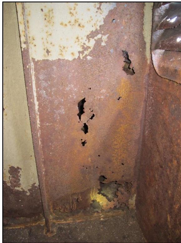
5 Figure 35. El Yunque , interior bulkhead of exhaust ventilation trunk holed from corrosion at frame 6 123, viewed looking forward. Bulkhead separates two forward and aft exhaust ventilation trunks 7 for hold 2. The holed plate depicted allows communication only between adjacent trunks to 8 sideshell louver openings. It is not through a baffle plate and does not permit water ingress directly 9 to exhaust ventilation trunks or into the cargo hold below. (Photo from September 2016)
