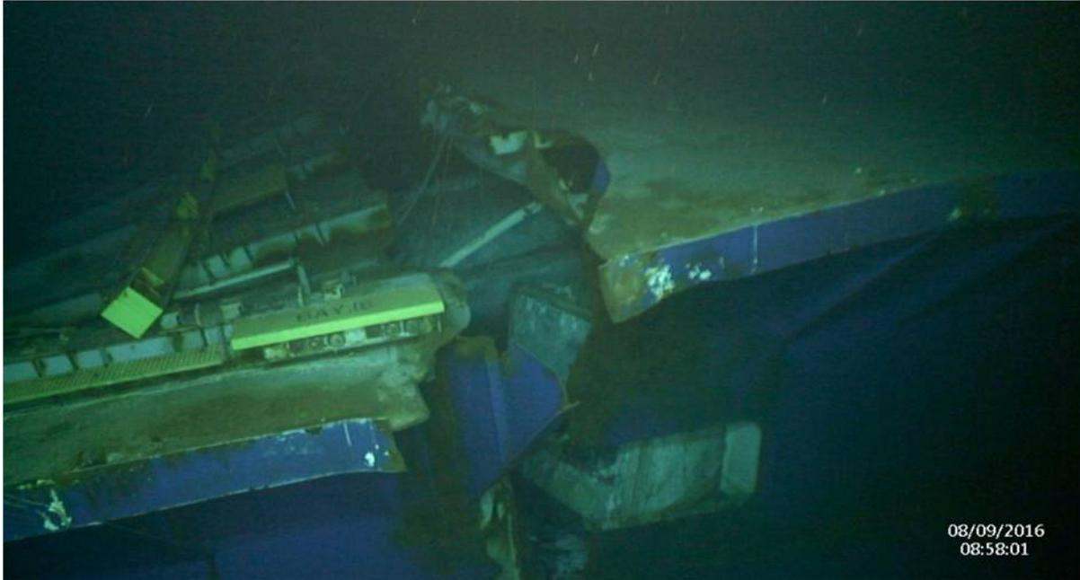
**Figure 6-7: Top Deck Edge View of Hull Crack at Bay 16 And Aft Engine Room Bulkhead**
