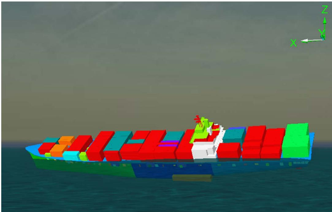
**Figure 7-1: El Faro Heeled Down with Wave / Green Water Over the Vent Openings**
