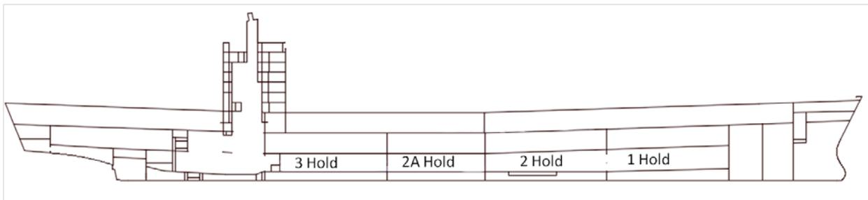
**Figure 3-8: Hold Labels Used on Bridge Audio**
