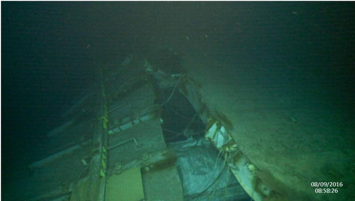
**Figure 6-8: View of Top Deck Showing Crack Traveling All the Way Across the Hull**
