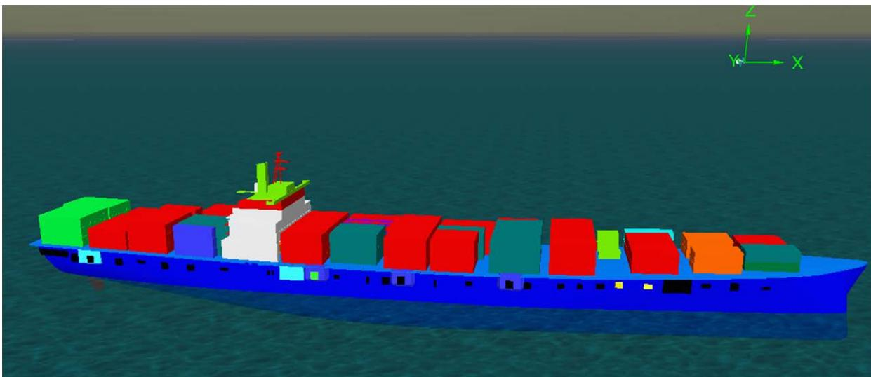
**Figure 2-4: OrcaFlex Model of EL Faro with Container Load and Hull Openings (early version)**
